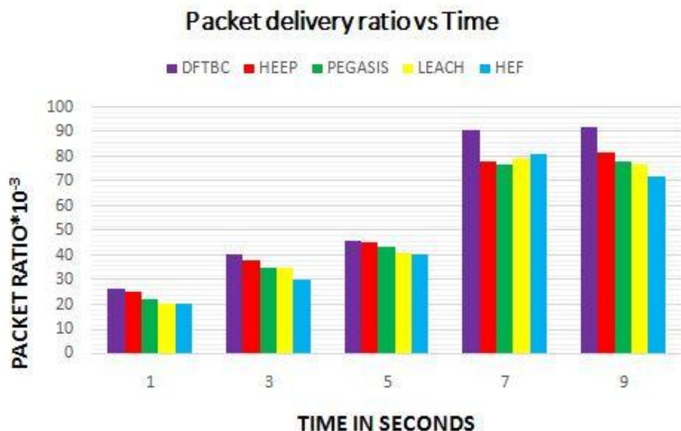
**Figure 2: Analysis of Packet delivery ratio Vs time**
